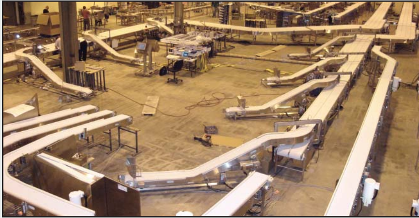
Large system set up for F.A.T. (Factory Acceptance Test).
