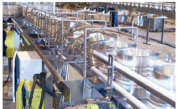
Nercon designs twist rinsing equipment that utilizes ionized air or water.
