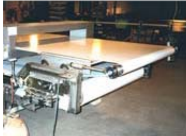
Nercon has vast experience conveying confectionery products on various belt systems such as this retractable noser conveyor.
