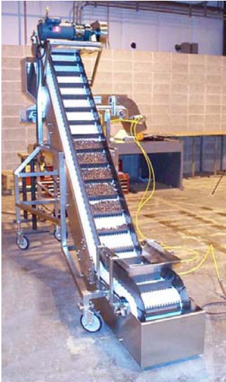
Sanitary design bulk elevator handling chocolate candy pieces.
