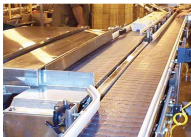
A 2 to 1 lane merge conveyor system, pushing slugs of sugar packages.
