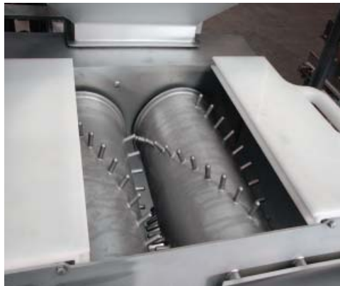
Cluster buster device designed to gently break up frozen clusters of frozen raw vegetables.
