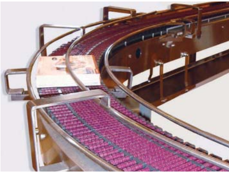
Frozen dinner sanitary design conveyor with easy guide rail positioning.
