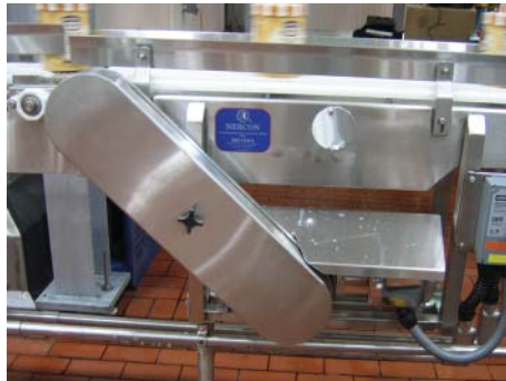
Closed top design frozen dairy process room conveyor.
