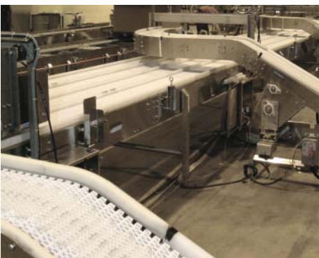
Mat-style system with multiple spurs handling frozen bagged appetizers.
