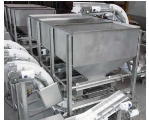
Hoppers, conveyors and devices are bead blasted, stainless steel, sanitary constructed.
