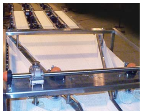
Servo merge with powered side belt handling meat trays.
