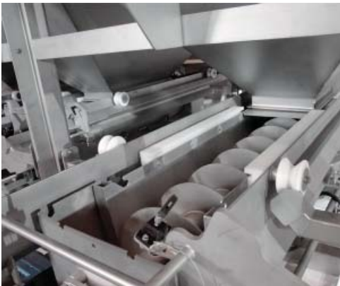
Reversing auger in pull-out full access position.
