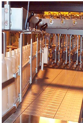
Nercon has engineered and manufactured a variety of laned conveyor systems as well as high speed merging conveyors for the health and beauty industry.
