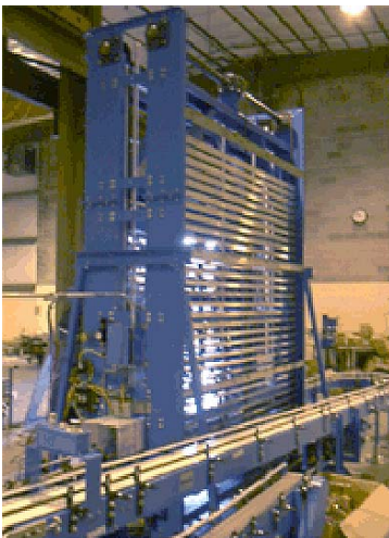
First-in, Last-out Vertical Accumulator designed to Accumulate rows of hair care carton packaging.
