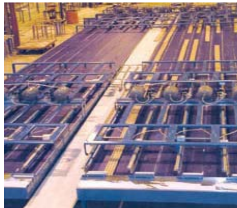
Nercon engineered and manufactured this cooling conveyor system to transport molded decking boards.
