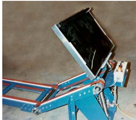
An ergonomic lift device used in appliance production.
