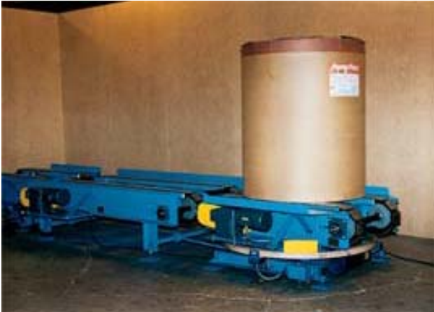
Nercon engineered this conveyor to weigh and scan bar codes on 3,000 lb. master paper rolls.
