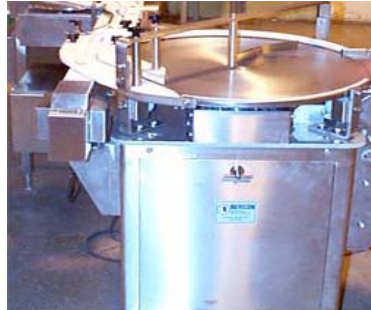
This rotary table single files small vials into the production line.
