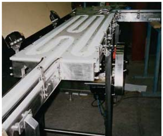
This serpentine accumulator provides cooling time for small vials of liquid medical products.
