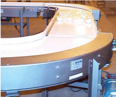
This powered belt curve conveyor is transporting wrapped bandages.
