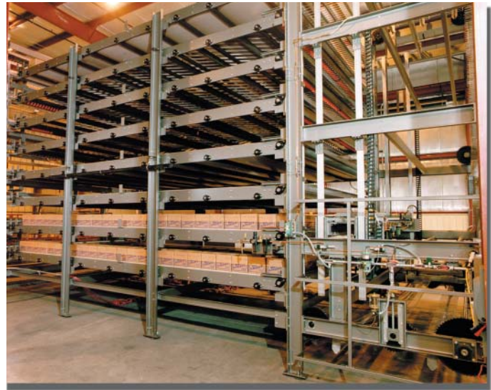
This case accumulation system is also effective when used to condition and age various products ranging from bread and cheese, to frozen dinners.
