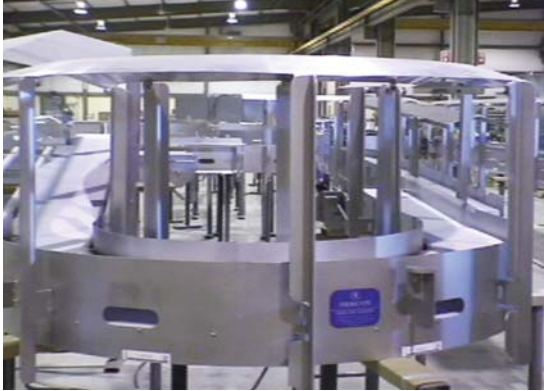
A version of our standard design, covers were added to this pie handling conveyor line.
