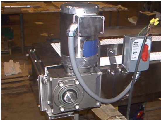
This shaft mounted stainless steel motor is temporarily wired for testing at Nercon's factory.
