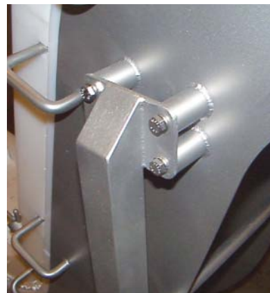
Welded stand-offs eliminate debris-catching crevices.
