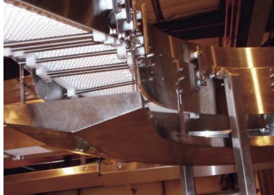
This sanitary conveyor features catch pans and off set, spaced square tube supports .
