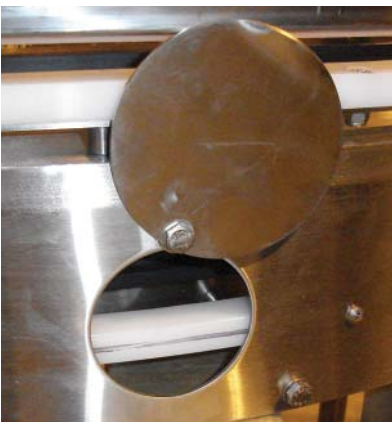
This access for cleaning opening has a pivoting safety cover .
