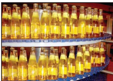
The Live Drum Spiral can conveyor various packages from bottles to totes.
