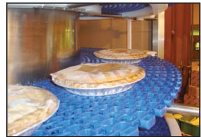
It can be designed as an elevator, lowerator, twin accumulator, ambient cooler or proofer.
