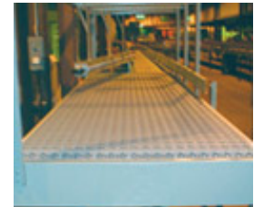
Angled roller top aligns multi-size cases to one side for code dating or bar code reading
