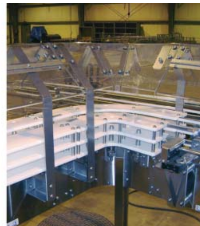
Guides can be specially designed out of UMHW; they are set in place on the conveyor when needed to run a particular product size.
