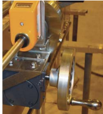
This hand wheel is integrated with the digital counter for fast and accurate rail adjustment.
