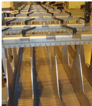
Ruler guides can be bolted-on for quick adjustment, or etched as shown here.
