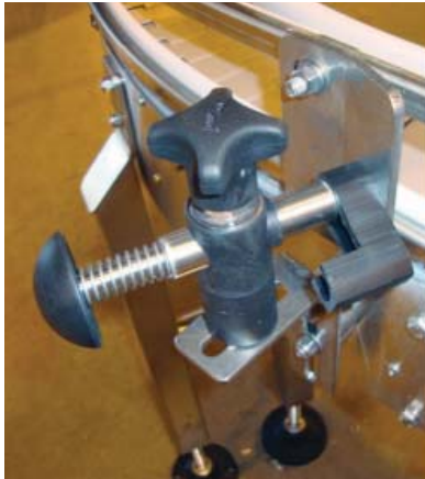
The quick set rail with hand knob, has a spring that pops in place on the pre-set adjustment.
